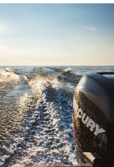
Figure 8. As motorised watercraft move through the river their hull displaces water, pushing a wave, or wake behind them. This wake breaks against the banks, with the force breaking down sediments - contributing to undercutting and instability.
