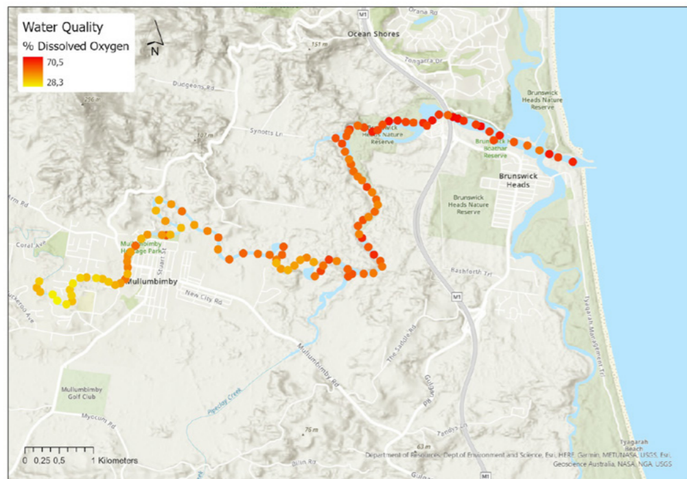
Figure 17. A snapshot of Dissolved Oxygen (DO) shows the shift from more oxygenated water from the ocean on a given tide, slowly decreasing upstream.
